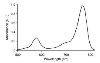
Figure I Absorption spectrum for a solution of bacteriochlorophyllserine in acetone.
