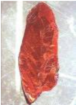
Thin slice after ammonolysis LaTiO 2 N
