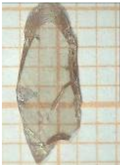
Thin slice of LaTiO 3.5 crystal
