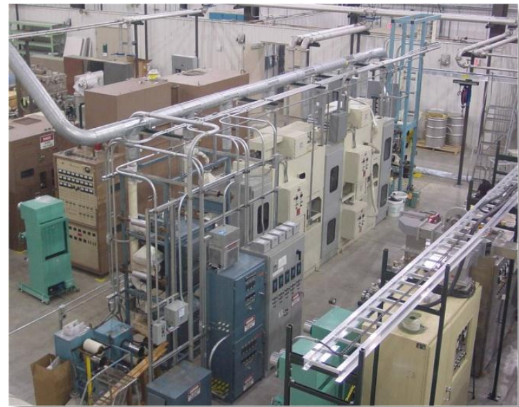
Pilot-scale, multiple-tow carbon fiber conversion line ( \approx 20 lb/day)
