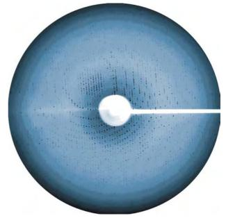
Fig. 2. A 1° rotation diffraction pattern obtained from a treated crystal of the small subunit from *Thermus thermophilus* (T30S) obtained at ID2/ESRF.
