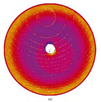
Fig. 1. Diffraction patterns  $(0.5^{\circ} \text{ rotation})$  obtained within 20 s at the microfocus beamline (ID13) at ESRF from a crystal of H50S soaked in solution with 0.5 m*M* of W30. (*a*) The first pattern; (*b*) after 3.5° rotation.
