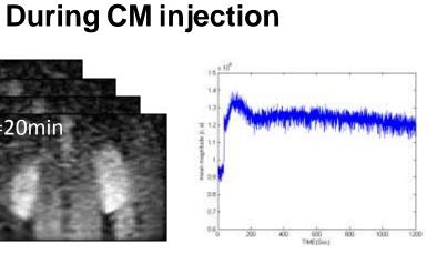
Fast kinetics of 2D SPEN of both Kidneys after Gd-DTPA injection. The plot describes the kinetics of only the kidney circled by ROI. The 2D SPEN with FOV of 30×30mm and voxel size of 0.3×0.3×2mm. Sequence duration of 50ms, recycling time of 250ms, 4000 repetitions for 20min.
