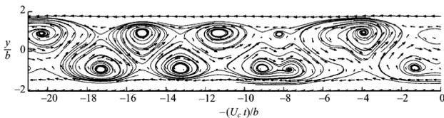
FIG. 2. Velocity field lines showing the vortex structure (a fragment from experimental proper orthogonal decomposition, Ref. [7]).
