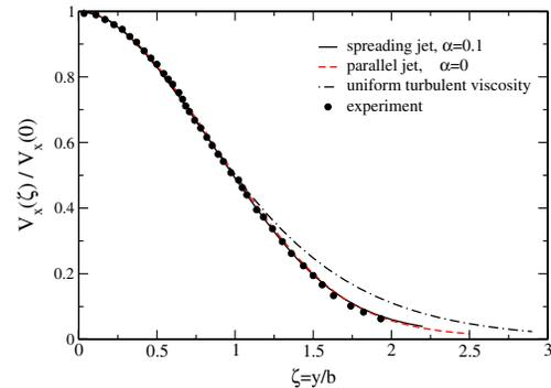
FIG. 1 (color online). Profiles of the normalized streamwise mean velocity: Black squares—experimental points [7]; black dashed line—profile (9) obtained from the Prandtl closure with constant turbulent viscosity approximation; red dash-dotted line—Eq. (7) ( $\alpha \rightarrow 0$  limit) with  $a = 0.747$ ,  $c \approx 1.1$ . Black solid line—profile (8) with  $\alpha = 0.1$  and the same values of  $a$  and  $c$ .
