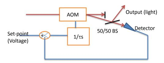
Acousto Optic Modulators are optical switches that diffract light into a given direction from a traveling acoustic wave that can be switched on or off.
