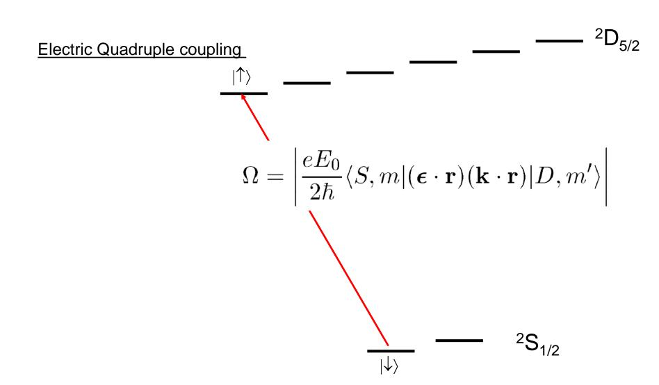
Optical qubit: Electric Quadruple coupling
