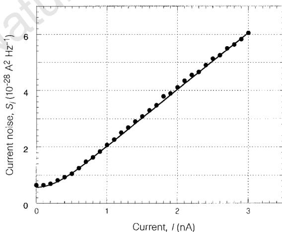
**Figure 2** Quantum shot noise as a function of direct current,  $I$ , through the QPC without an applied magnetic field (circles). The solid line is equation (2) with the temperature (57 mK) deduced from Fig. 1. The transmission,  $t$ , is 0.37.
