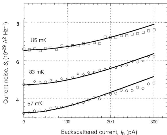
**Figure 4** Quantum shot noise as a function of backscattered current,  $I_B$ , in the FQH regime at  $\nu = \frac{1}{3}$ , for three different temperatures and a constant transmission coefficient,  $t = 0.8$ , through the QPC.
