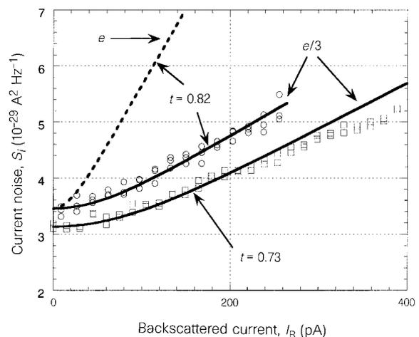
**Figure 3** Quantum shot noise as a function of the backscattered current,  $I_B$ , in the FQH regime at  $\nu = \frac{1}{3}$  for two different transmission coefficients through the QPC (circles and squares). The solid lines correspond to equation (2) with a charge  $Q = e/3$  and the appropriate  $t$ . For comparison the expected behaviour of the noise for  $Q = e$  and  $t = 0.82$  is shown by the broken line.
