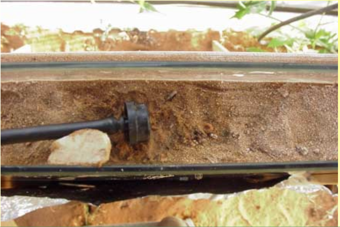
Normal ponded area in sand irrigated with fresh water
