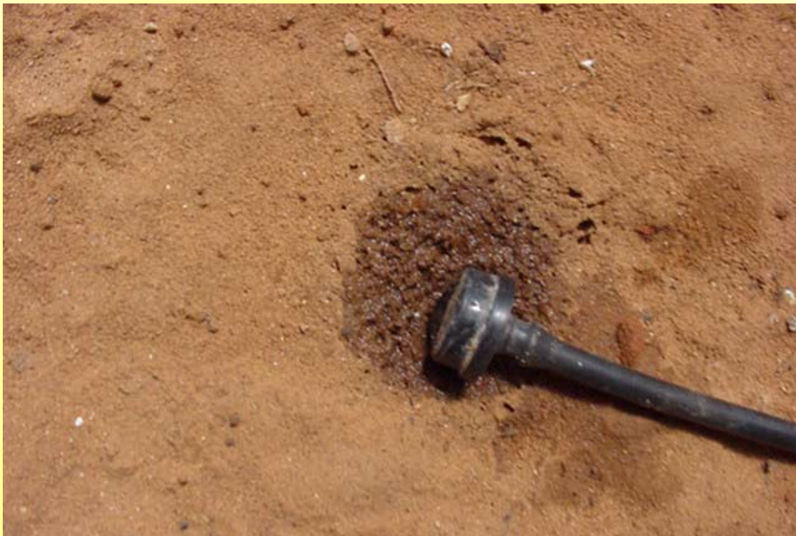
Disappearance of the ponded area in sand irrigated with effluents (after 30 seconds)
