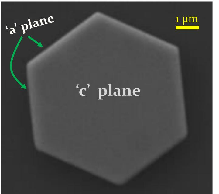
Dipping in o.1M CH<sub>2</sub>NH<sub>2</sub>I in IPA for 55 hours (@RT)
