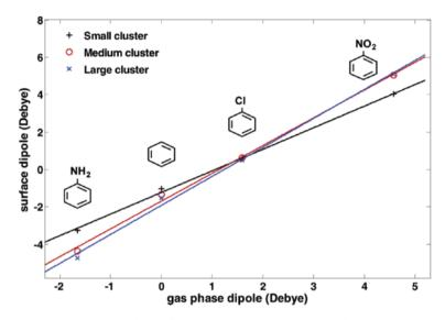
Fig. 6. Same as Fig. 5 for a single molecule adsorbed on silicon clusters of different sizes. <sup>19</sup> Using linear regression, slopes of 1.15, 1.48, and 1.55 are found for the "small" (1 atom), "medium" (14 Si atoms), and "large" (38 Si atoms) clusters, respectively.
