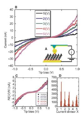
Fig. 1. Conduction of 1,8-octanedithiol molecule in the configuration shown in A. (after Cui et al<sup>2</sup>). Several conductance characteristics (B) collapse into a single line following scaling by intergers from 1 to 5 (C). D shows an histogram of conductance signals.
