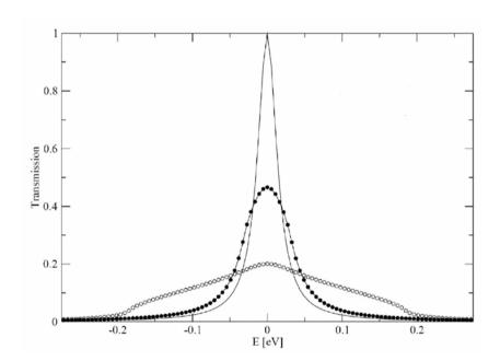
Fig. 8 White circles: Transmission (per molecule) as function of energy through a ML, calculated with model parameters  $V^{(t)} = 0.03$ a.u.~0.82 eV,  $V^{(m)} = 0.0035$  a.u. ~ 0.095 eV,  $V^{(mt)} = 0.004$  a.u. ~ 0.11 eV and
