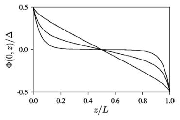
Figure 4. The potential profile along a molecular wire computed from Eqs. (3) - (6) is shown for a screening length  $\lambda/L = 0.05$ . The thickness parameter  $\sigma/L$  takes the values 0.0125, 0.05, and 0.5 from the almost linear behavior to the voltage profile containing almost a plateau. From Nitzan et al. <sup>13</sup>
