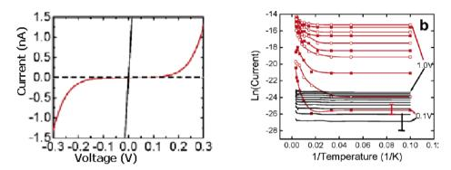
Fig. 2. Conductance of 1-nitro-2,5-di(phenylethynyl- 4'-mercapto) benzene between gold leads. Left: Red – single molecule; black – molecular layer. Dashed black is the molecular layer signal normalized per molecule. Right: Temperature and voltage dependence of conduction. Red – single molecule; black – molecular layer per molecule. From Selzer et al<sup>7</sup>.
