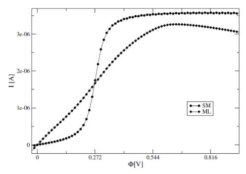
Fig 9. Current I (per molecule) as function of the bias voltage  $\Phi$  via a SM (circles) and ML (diamonds), with the molecular level set at  $\varepsilon_m = -0.136 \text{eV}$ .  $\varepsilon_t$ , taken as the energy origin is also the Fermi energy in this
