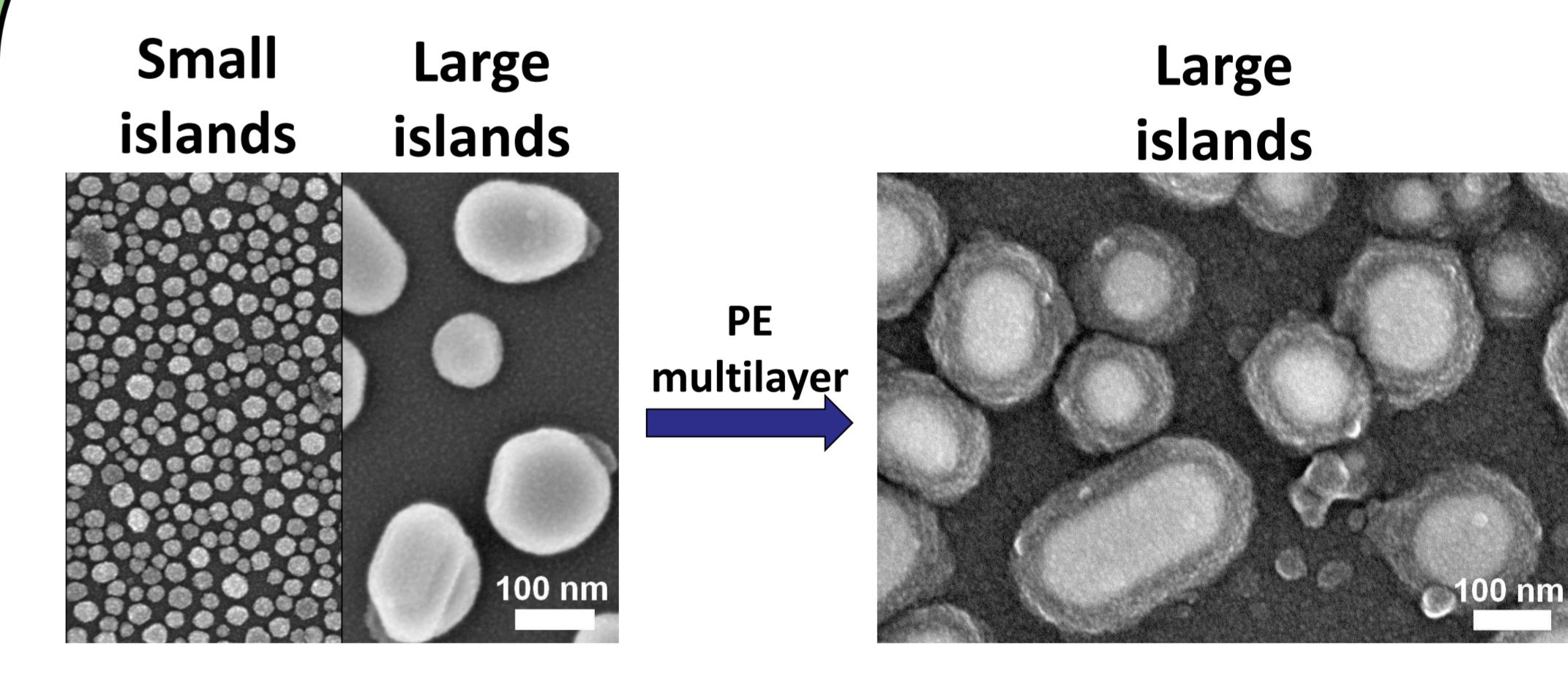
High-resolution SEM images of Au island films thermally evaporated on glass slides and annealed 10 h at 580 °C. Left: samples of 3 nm and 10 nm nominal thickness; right: 10 nm (nominal thickness) islands, coated with 40 polyelectrolyte layers. In-Lens SE detector, 10-20 kV; coated with 2-3 nm Cr.
