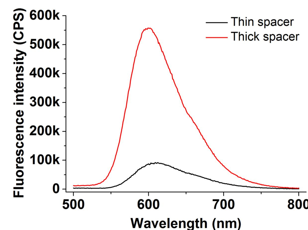
For thin spacers, the fluorescence is strongly quenched. Fluorescence intensity on large islands, for spacer layers 2.1 nm and 44.1 nm thick.
