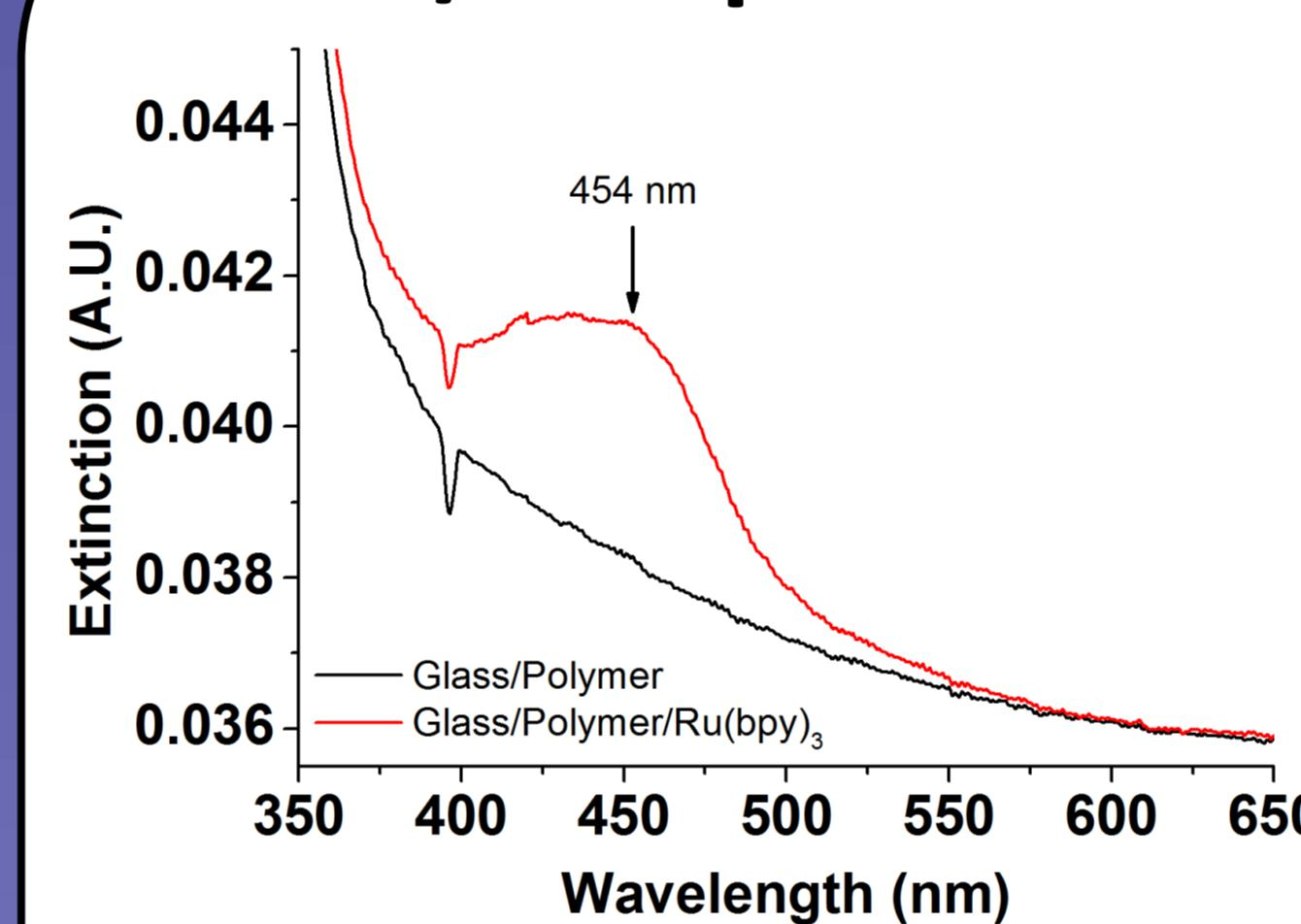
Peak intensity varies by <20% for 9 slides, showing the repeatability of the adsorption method.
