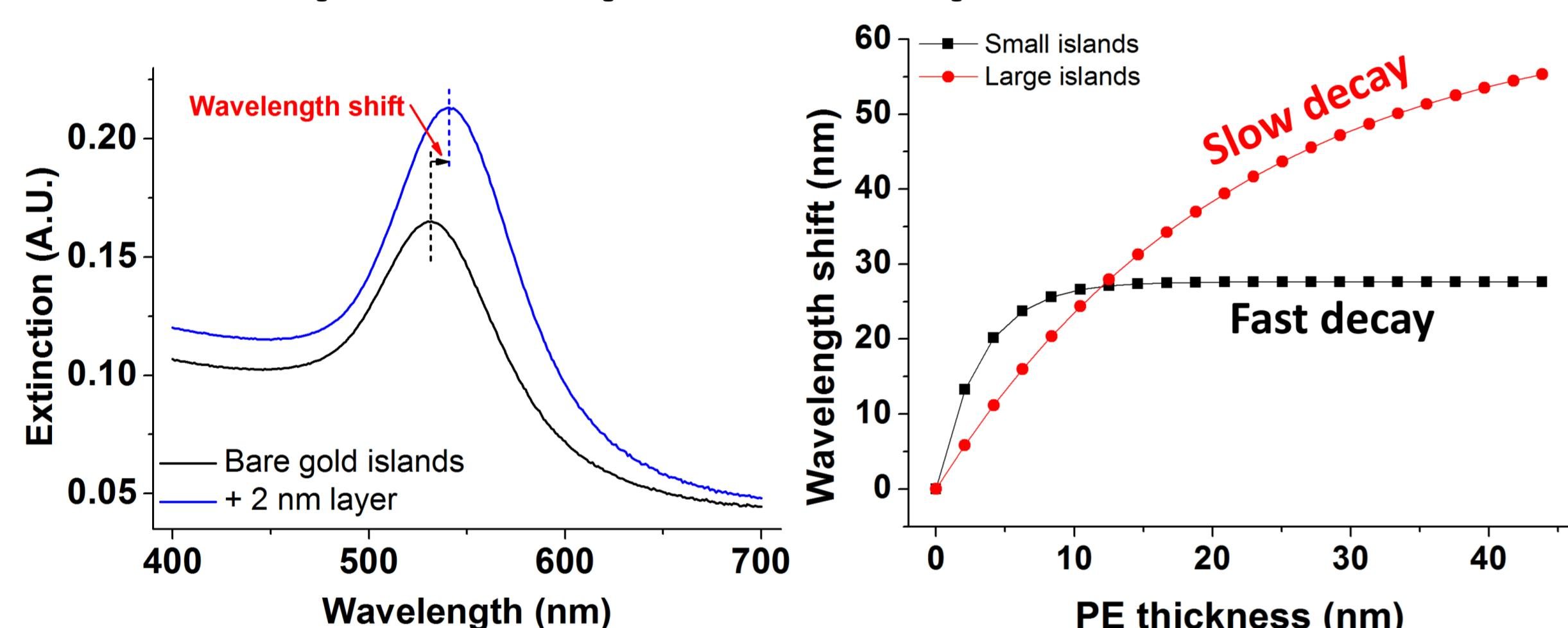
Shift of the LSPR peak wavelength upon adsorption of a dielectric layer of increasing thickness. The response decays rapidly for small islands (no change after ~10 nm) and slowly for large islands (the peak shifts even after 40 nm).
