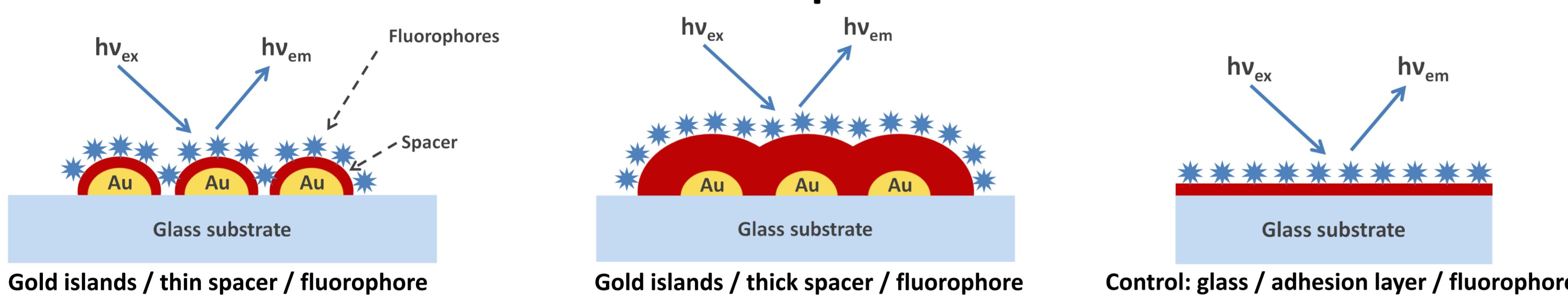
Two types of Au nanoisland films were used, of ~20 and ~100 nm average diameter. Fluorescence intensity measured as a function of metal-fluorophore separation, compared to intensity from fluorophore on inert substrate as a control.
