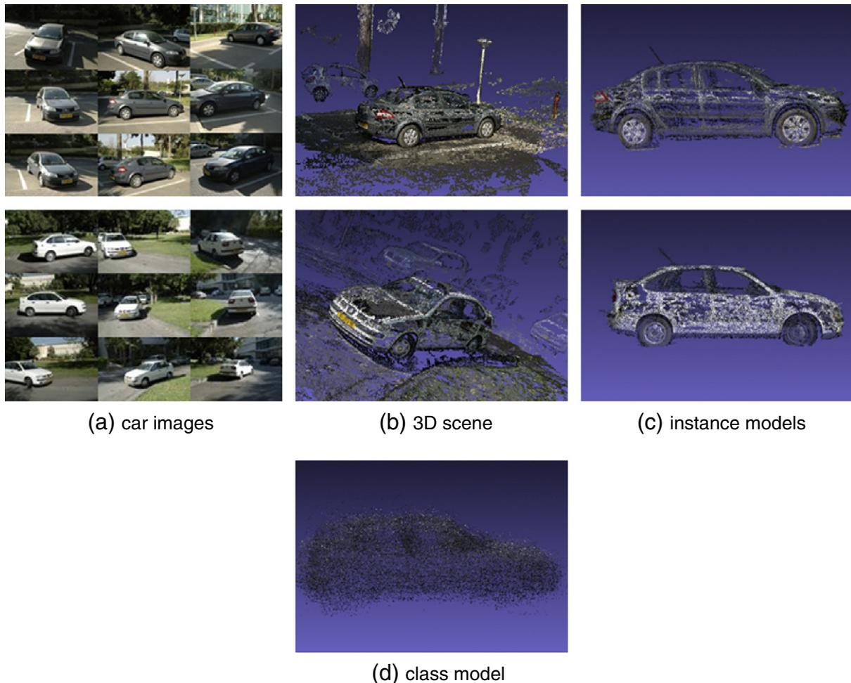
**Fig. 4.** Model construction. We construct the model from multiple sets of car images, some example frames from two different sequences can be seen in (a). Using Bundler we re-construct a 3D scene (b). The car of interest is manually segmented and aligned (c). Finally a view of the class model is shown in (d).
