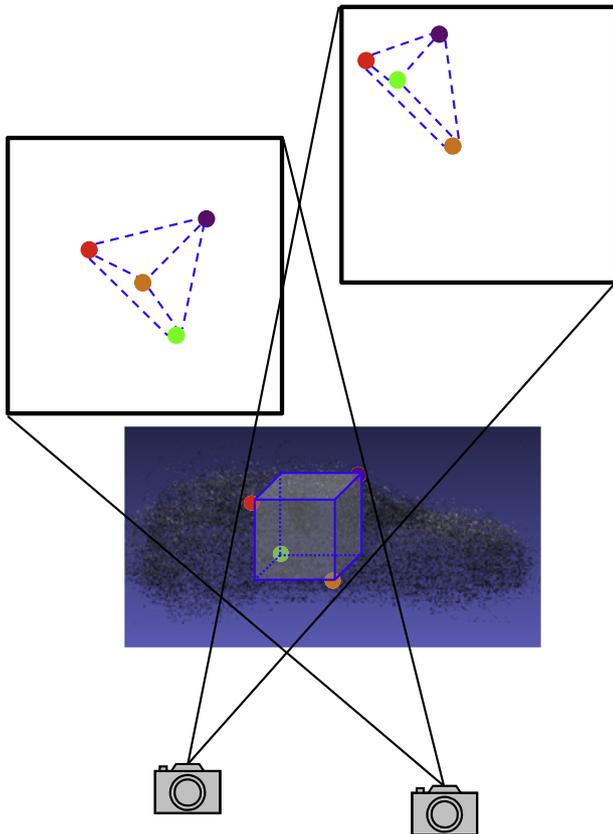
**Fig. 2.** Parameterization. We suggest to parameterize the 6 DOF transformation which relates the 3D model to an instance in a 2D image by the action of the transformation on a set of 4 fixed designated points. The 4 designated points are shown, superimposed over the 3D model. Different cameras project the points to different locations in the image plane. The concatenation of the coordinates of these projections defines our 8 dimensional representation.
