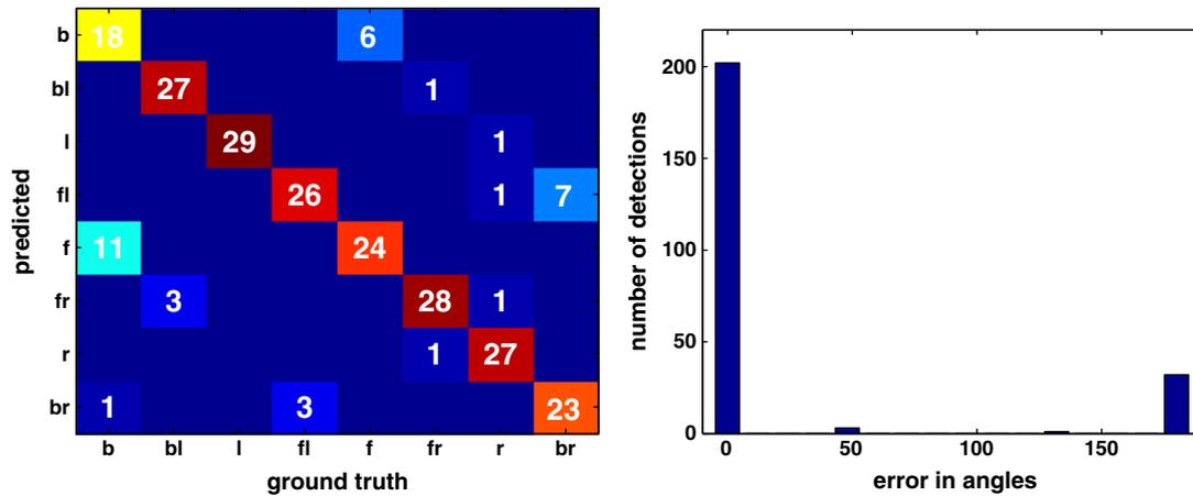
Fig. 7. Stanford 3Dpose cars – pose estimation. A confusion matrix and a histogram of label differences. Average accuracy is 85.28%.
