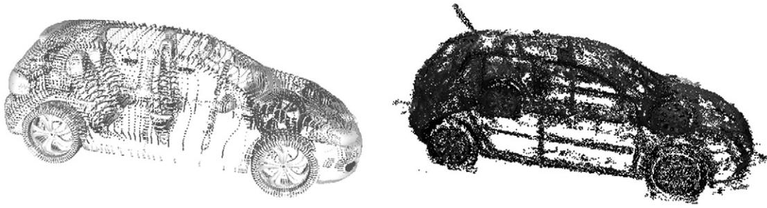
Fig. 5. Comparing CAD and SfM. We compare a CAD model (left) to the point cloud reconstructed using [2] and [3]. Using ICP we align the two models and measure the errors. The median error is 1.6 cm, less than one percent of the car's width.
