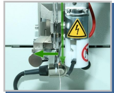
move clamp aside and pull wire through glass tube
