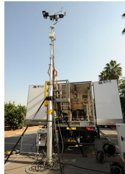
Fig. 2. Measurement mobile system. Measuring components (left) installed on top of the mast: Sonic 3D anemometer, Li-7200 IRGA, six radiation sensors (PAR, long and short wave, up and down) and meteorological hut (air temperature and humidity). The mast opened next to the mobile lab (right bottom).
