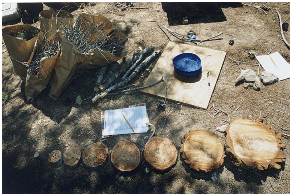
Figure 1. Subsampling stem sections and branches for moisture content during a field campaign aimed at creating site-specific allometric equations for Pinus halepensis (picture courtesy: Avi Bar Masada).
