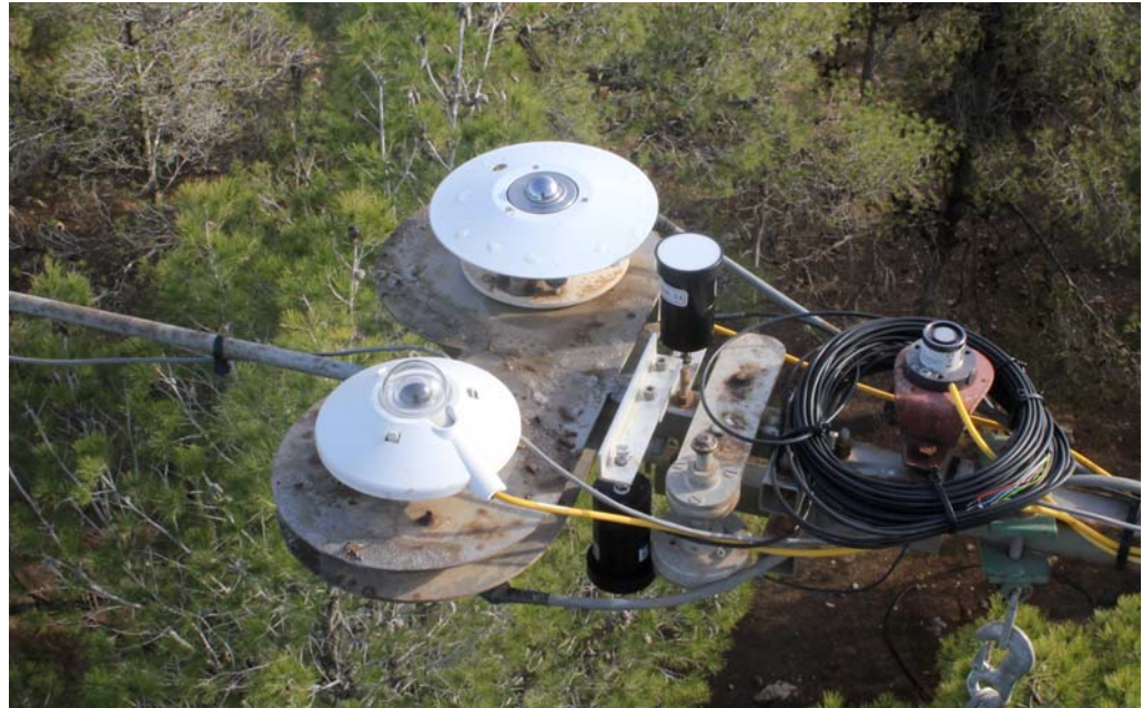
Figure 2: The radiation measurement setup over the Yatir forest, included: 2 - Kipp&Zonen CM21 for the solar radiation range, 2 - Eppley PIR for the thermal range, 2 - Kipp&Zonen PQS1 for the PAR and 2 - Skye 4 Channel SKR 1850 sensors. A set of sensors is looking upward (to the atmosphere) the other downward.
