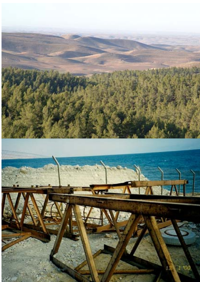
Figures 1&2. Yatir Forest (above) and an old building construction crane converted to a flux tower (below).
