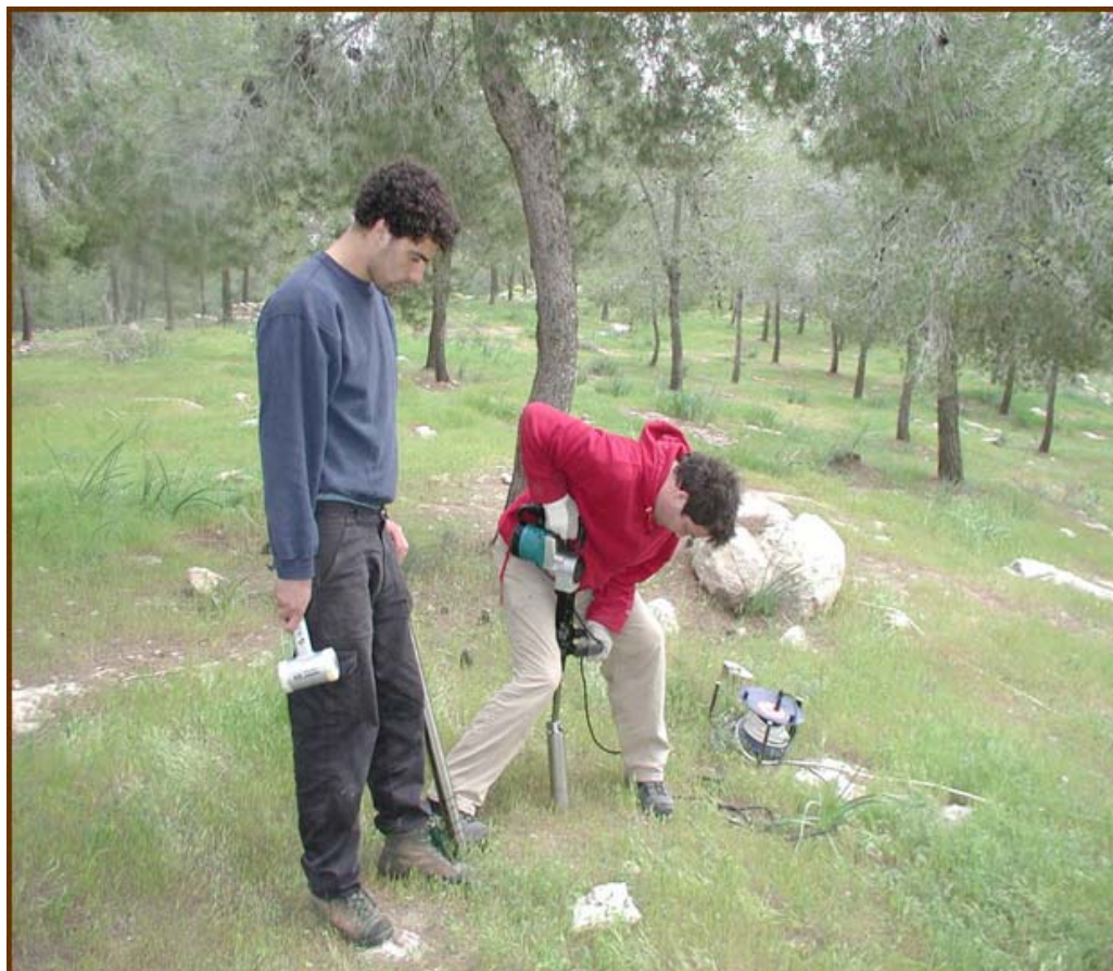
Figure 2. Ilya Gelfand and assistant coring soil in Yatir for nitrogen analyses and for seasonal incubations
