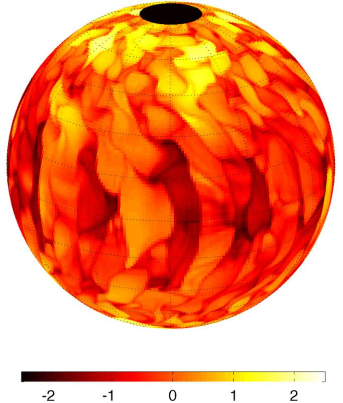
**Figure 5.** Temperature variations at 1 bar in a typical, rapidly rotating brown-dwarf model. The colorscale gives the temperature perturbation  $T'$  at 1 bar, that is, the deviation of temperature from its reference value. Rotation period is 10 hr. (A color version of this figure is available in the online journal.)
