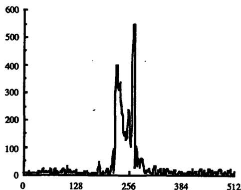
**Figure 2** The S/N improvement possible using multiple  $90^\circ$  pulses to hold up the magnetization.
