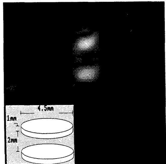
Figure 1 Two-dimensional proton density map of two red rubber discs as shown in the inset obtained by method 1 as described in the text.
