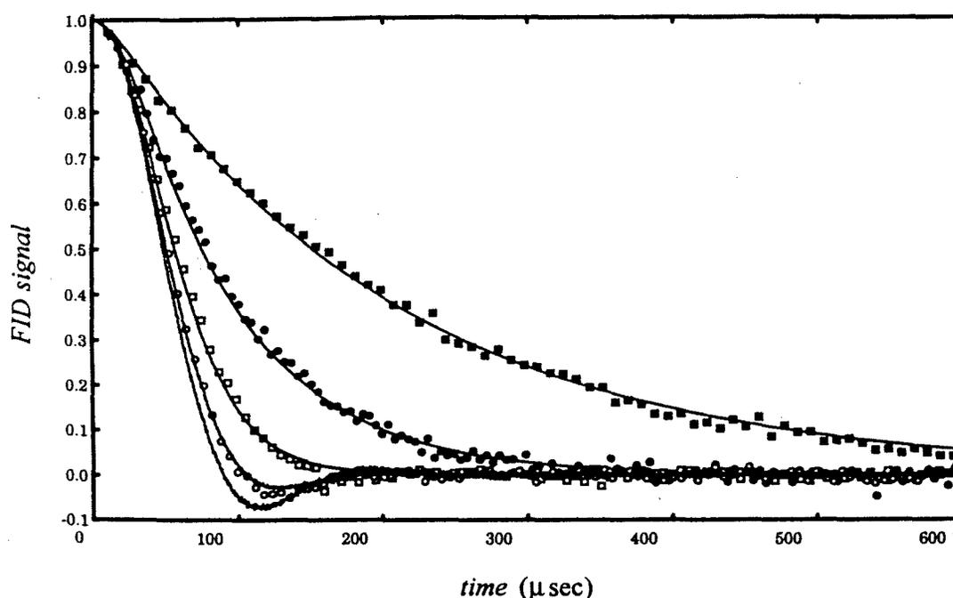
figure 1: Free Induction Decay Signals at different temperatures: open circles: 283 K, open squares : 292.5 K, full circles: 303 K, full squares : 311.3 K. Solid curves are calculated with our model.
