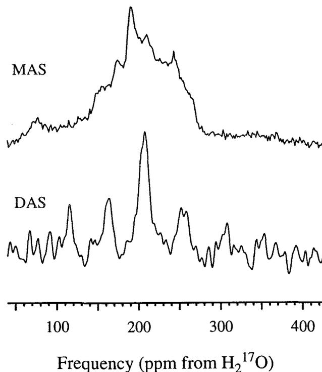
Figure 3: Magic-angle spinning (MAS) and dynamic-angle spinning (DAS) spectra of  $^{17}\text{O}$  in L-alanine at 11.7 T (67.797 MHz), without proton spin decoupling. The spectra are referenced to  $^{17}\text{O}$  labeled  $\text{H}_2\text{O}$ .
