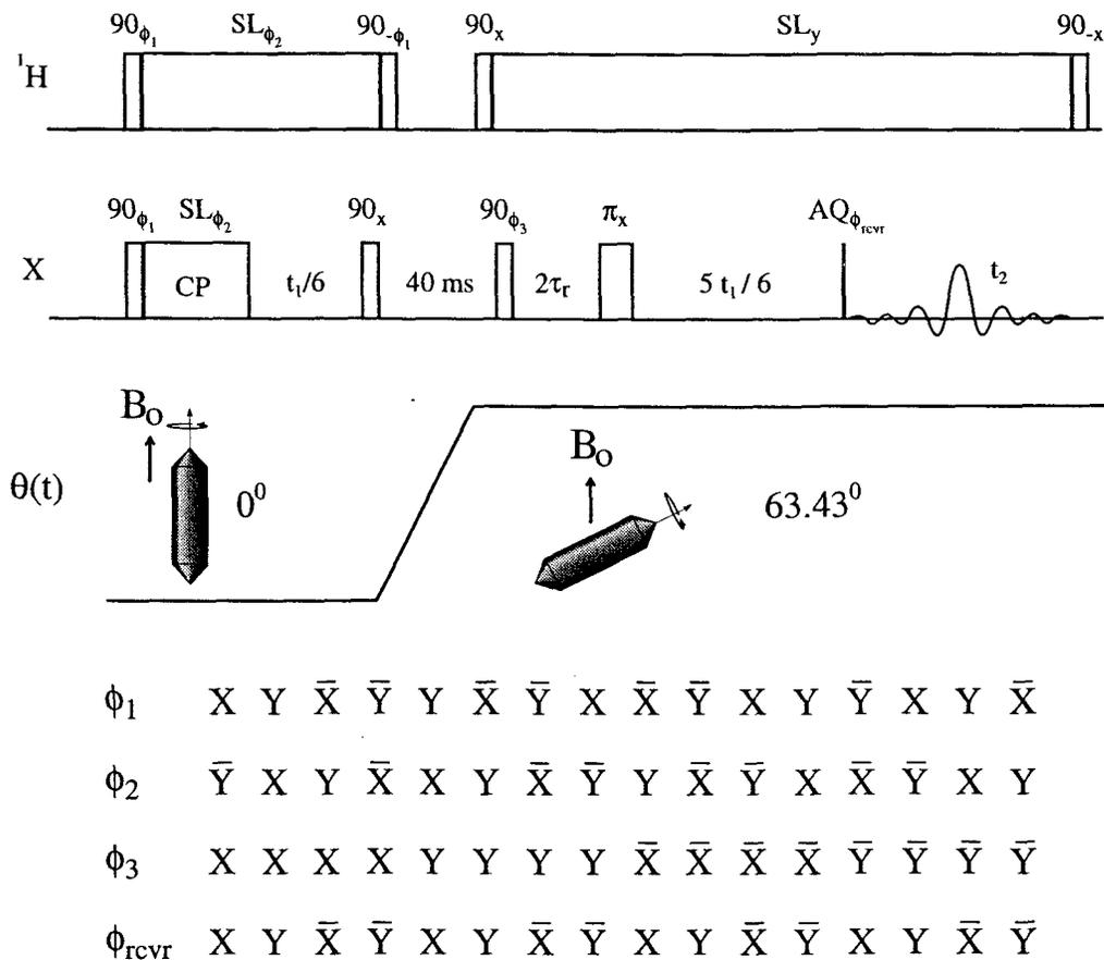
Figure 1: Pulse sequence and phase cycle for dynamic-angle spinning with cross-polarization (CP/DAS). SL signifies spinlock/decoupling and  $\tau_r$  is the rotor period.
