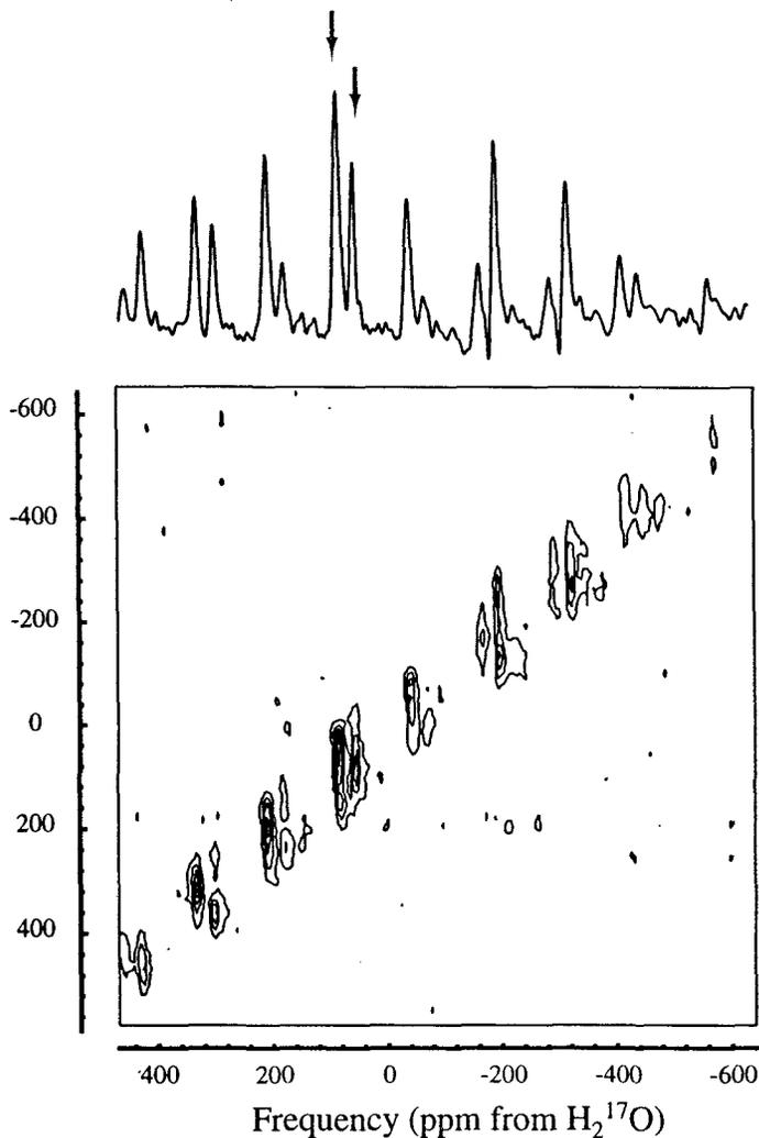
Figure 4: Two-dimensional DAS with cross polarization (CP/DAS) and proton spin decoupling spectrum of  $^{17}\text{O}$  in L-alanine at 7.04 T. The projection of the isotropic shift dimension is shown at the top. The spectrum is referenced to  $^{17}\text{O}$  labeled  $\text{H}_2\text{O}$ .
