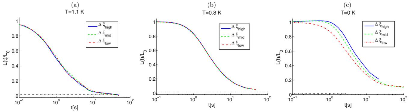
FIG. 4. (Color online) (a)–(c) Comparison of the time dependence of the normalized mean VLD  $\langle \mathcal{L}(t)/\mathcal{L}_0 \rangle$  for different resolutions and for  $T = 1.1$  and  $0.8$  K and  $T = 0$ . The horizontal dashed-dotted red line shows the background VLD  $\mathcal{L}_{\text{bg}} = 100 \text{ cm}^{-2}$ .
