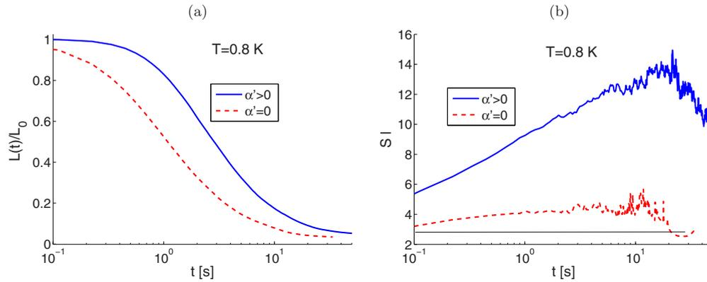
FIG. 7. (Color online) Comparison of the evolution of the normalized VLD  $\mathcal{L}(t)/\mathcal{L}(0)$  (a) and of the normalized curvature  $S(t)/\ell(t)$  (b) for the simulations with  $\alpha = 6.49 \times 10^{-4}$  and  $\alpha' = 4.635 \times 10^{-4}$  (corresponding to  $T = 0.8$  K, see Table I), shown by solid blue lines, and with the same  $\alpha = 6.49 \times 10^{-4}$ , but  $\alpha' = 0$  (dashed red lines).
