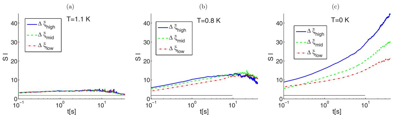
FIG. 5. (Color online) Comparison of the time dependence of the normalized curvature  $\ell(t)\tilde{S}$  for different resolutions and the same temperatures.
