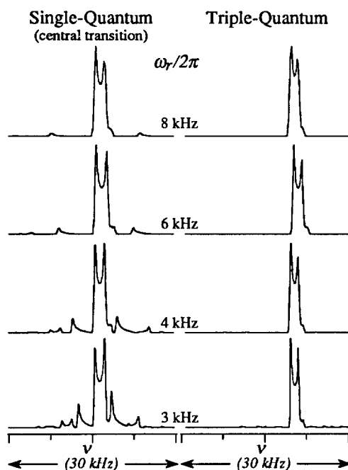
Fig. 2. Variable spinning speed simulations of idealized single- and triple-quantum MAS line shapes arising from a spin- 3/2 powder in the presence of second order quadrupole effects. The parameters employed in these calculations correspond to an on-resonance ^{23}\text{Na} site at 4.7 T with a coupling constant e^2qQ/h = 2.6 MHz and an asymmetry parameter \eta = 0 .
