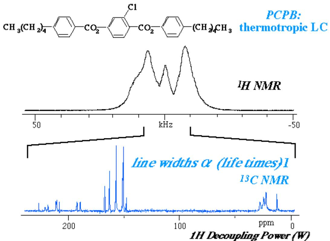
As shown by these CPMG spin-echo measurements, an important consideration in these liquid crystal NMR experiments is **the level of  $^1\text{H}$  decoupling**: the higher the field, the longer the FID
