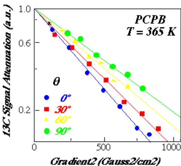
$^{13}\text{C PGSE decay curves of PCPB resonances as a function of gradient orientation}$
