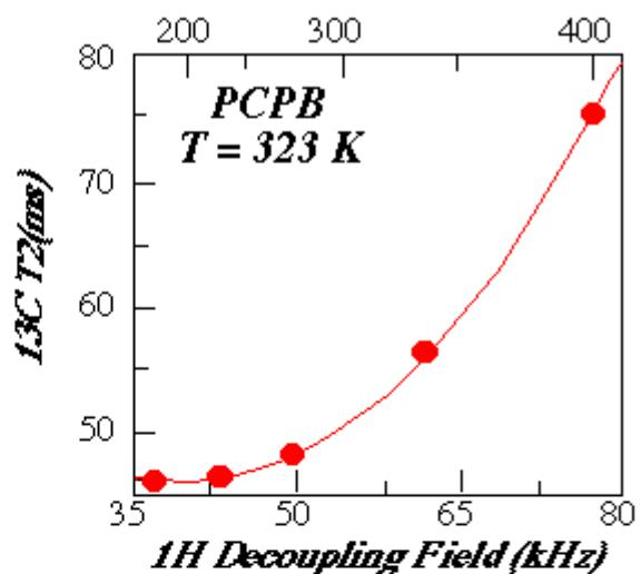
Appropriate decoupling levels enable the PGSE measurement of diffusion coefficients in these phases:
