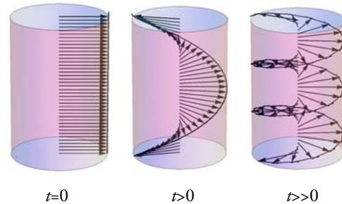
In the presence of a z-gradient, the spins precess with a frequency  $\omega = \gamma Gz$  which induces a linear phase  $\phi(t) = \gamma Gzt$ , imparting a helical shape to the tips of the magnetization vectors as time progresses.
