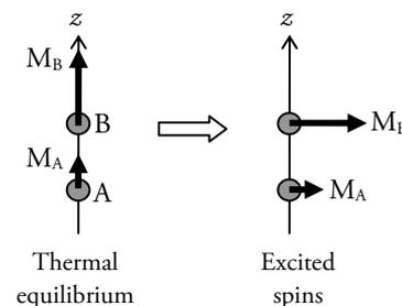
By exciting and acquiring, the signal we would measure would originate from both points equally, and would lack any spatial selectivity:
