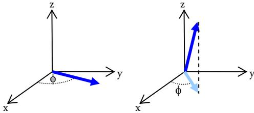
Left: the phase of a spin in the xy-plane is the angle it makes with the x-axis. Right: for a spin not in the xy-plane, one examines the phase its projection on the xy-plane makes with the x-axis.
