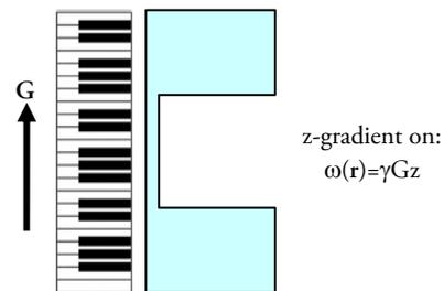
The intensity we "hear" at frequency - at each piano key - is proportional to the number of spins at that position. Therefore, by "listening" to the signal we can deduce the distribution of spins along the  $z$ -axis. This is the basic idea behind frequency encoding. The image obtained would give us a **projection** of the density of spins on the  $z$ -axis:
