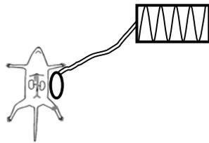
By placing a coil close to the rat's kidney, one can pick up signal mostly from the kidney where  $B_{rec}$  is strongest.
