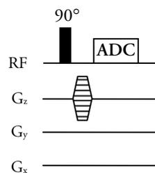
The striped gradient shape indicates that is a phase encoding gradient, which should be incremented by some fixed amount between successive phase encoding steps.
