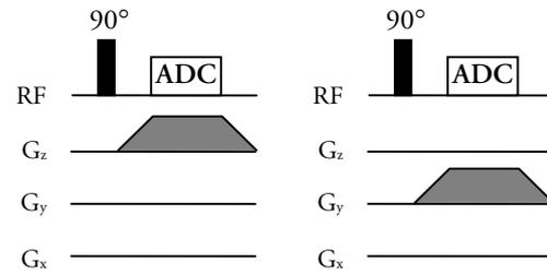
Left: pulse sequence depicting a volume excitation of the entire sample (i.e. not a slice selective excitation), followed by frequency encoding along z. Right: same sequence, only with frequency encoding along y.
