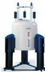
The sole purpose of the spectrometer is to generate a large and very stable and homogeneous magnetic field, denoted  $B_0$ . The purpose of this field is to polarize the nuclear magnetic moments, creating a macroscopic magnetic moment which can then be detected using methods we’ll discuss below.
