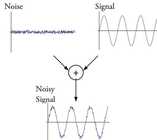
The signal to noise ratio of the noisy signal is defined as:
