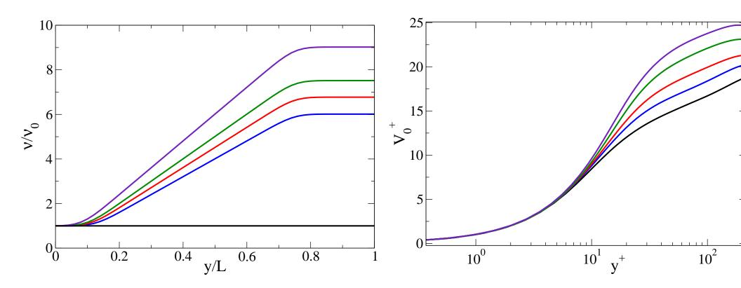
The viscosity (Left) & NSE-DNS mean velocity profiles (Right).  $\mathcal{R}e=6000$  (with centerline velocity). Solid black line — standard Newtonian flow. One sees a drag reduction in the scalar mean viscosity model.
