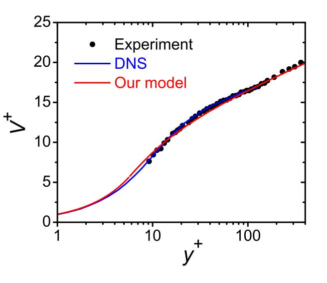
**Summary:** simple Our Algebraic Reynolds-stres model, based on the exac mechanica of balance momentum and K41 in spired model equation fo the local energy balance gives physically transparent analytical, semi-quantitative description of turbulen boundary layer
