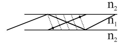
In considering the mode structure of waveguides we must solve for a self-consistent (phase matched) solution for a plane wave propagating at an angle to the waveguide. In doing this we have to take into account the phase shift following total internal reflection (remember polarization, beginning of semester).
