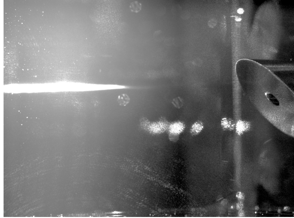
Figure 3.2: Side view of our ^{87}\text{Rb} 2D MOT by an IR camera. The shiny elongated glow on the left part is the 2D MOT fluorescence. On the right side the tip of the differential pumping tube with its 2 mm hole is shown.
