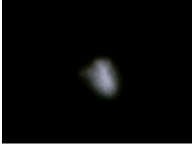
Fig. 9: A representative fluorescence image of the MOT. The CCD camera images the photons (wavelength of 780nm ) scattered by the atoms in the presence of the MOT beams.
