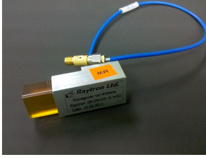
Figure 22: A compact microwave waveguide antenna used for injecting 6.8GHz radiation into the vacuum chamber.
