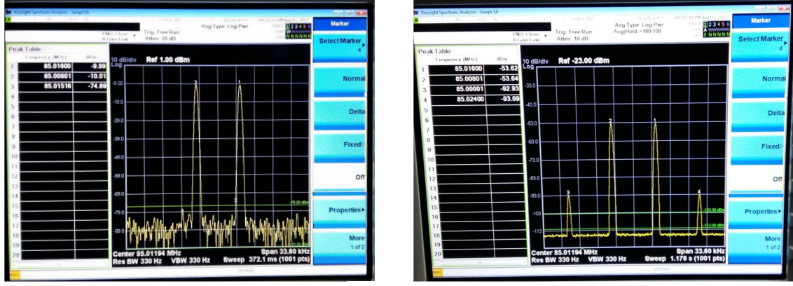
Figure 33: Example of 3rd order non linear signature of RF amplifier. Left: Spectrum of the blue side of the RF modulating signal for the Cardioid (1,2) measured after combining 4 DDS signals and before amplification. In this example we have \omega + \nu = 85 MHz and \xi = 0.008 MHz (these numbers were chosen arbitrarily), such that we observe \omega_{b_1} = \omega + \nu + \xi_0 as the left peak and \omega_{b_2} = \omega + \nu + 2\xi_0 as the right peak, both with an amplitude of \sim -10 dBm. Right: Same spectrum as but measured after RF amplification. Two new components appear: \omega_{3,1} = 2\omega_{b_1} - \omega_{b_2} = 85 MHz (left-most), and \omega_{3,2} = 2\omega_{b_2} - \omega_{b_1} = 85.024 MHz (right-most) which are 40dBm lower than the original driving fields. We note that \omega_{3,1} = \omega + \nu and thus creates on resonance blue side-band excitations.
