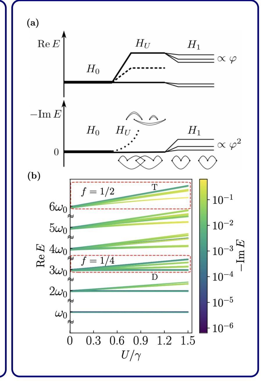
$$H = \omega_0 \sum_{j=1}^N \sigma_j^\dagger \sigma_j + \frac{U}{2} \sum_{j=1}^N \sigma_j^\dagger \sigma_j (\sigma_j^\dagger \sigma_j - 1)$$
