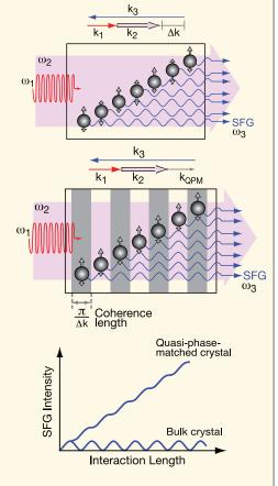
The difference between the incoming and outgoing wave vectors is usually termed the phase mismatch, denoted  $\Delta k$ , and the typical length over which a  $\pi$  phase shift is accumulated is called the coherence length. The value of the coherence length is typically just a few microns up to a few tens of microns for nonlinear interactions in the visible and
