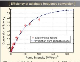
Efficiency of adiabatic frequency conversion for SFG of a signal beam  $(\omega_1)$  centered at 1,530 nm and a strong pump beam  $(\omega_2)$  centered at 1,064 nm. The maximum demonstrated conversion efficiency was 74 percent, but it can approach 100 percent using higher pump intensities. The analogy with other two-level systems enables analytic calculation of the expected conversion efficiency.
