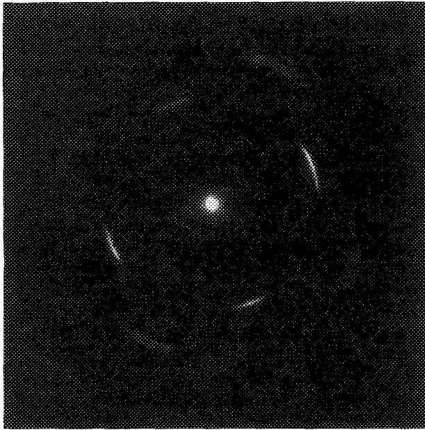
FIG. 5. Transmission electron diffraction pattern of Nb film, prepared at T_s = 170^\circ\text{C} and subsequently annealed at 440^\circ\text{C} for a few minutes, resulting in the formation of aligned NbAs.
