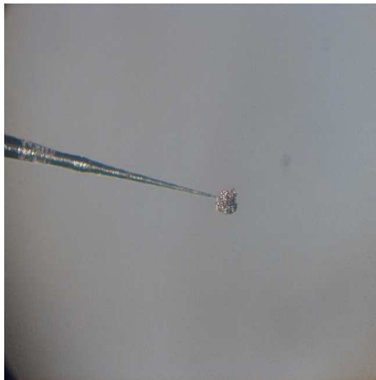
Fig. 3.4: Grown nickel on the end of a platinum wire tip.
