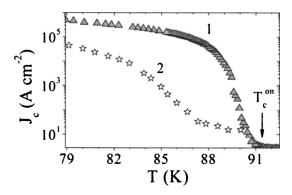
FIG. 4. Temperature dependence of the critical current density for a reference bridge (1 - triangles) and a bridge containing a single LW channel (2 - stars).
