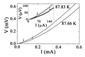
FIG. 5. V-I curves of a single-channel bridge at T=87.66 and 87.83 K in zero applied field. The arrows mark an onset of the Josephson-like step structures. Inset: low voltage part of the I-V curves on the expanded scale.
