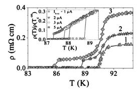
FIG. 3. Resistivity vs temperature dependences of a 50- $\mu$ m-wide and 100- $\mu$ m-long YBCO bridge with a single 5- $\mu$ m-wide LW channel (2 - stars) and with two LW channels separated by 10  $\mu$ m (3 - diamonds), measured with a dc current of 1  $\mu$ A. Curve (1 - triangles) was recorded for a channel-free reference device. The inset shows evolution of the resistive tail with changing dc current for a single-channel device.
