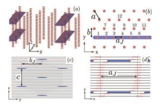
Fig. 1: (Colour on-line) (a) Schematic 3D plot of the crossing PV-JV lattice. The JVs are aligned along the x-axis and are stacked along z forming "Josephson planes" along xz-planes. (b) Top view (xy-plane) of the PVs (red) and JVs (blue). The vortex numbers are used in figs. 2 and 3. (c) Front view of the JV lattice (yz-plane). (d) Side view of PVs and JVs in the Josephson plane (xz-plane).
