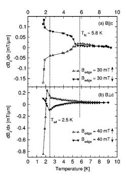
FIG. 3. Field gradient  $\partial B_z/\partial x$ , vs temperature for increasing (open symbols) and decreasing (closed symbols) field cycles at constant edge field,  $B_{edge}$ , for (a)  $\mathbf{B}\|c$  at 30 mT (triangles: Dewhurst  $et~al.^{14}$ ; squares: this work) and (b)  $B_5$ - $B_6$  at 40 mT for  $B\perp c$  (this work).
