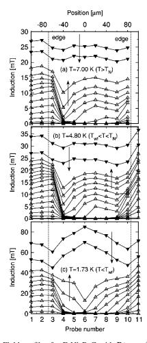
FIG. 1. Field profiles for  $\text{ErNi}_2\text{B}_2\text{C}$  with  $\mathbf{B}\perp c$  at (a) 7.0 K ( $T > T_N$ ), (b) 4.8 K ( $T_{wf} < T < T_N$ ), and (c) 1.73 K ( $T < T_{wf}$ ), for increasing (open symbols) and decreasing (solid symbols) applied field.
