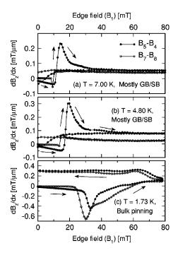
FIG. 2. Field gradient  $\partial B_z/\partial x$ , vs edge field  $\mathbf{B}_1$  at (a) 7.00 K, (b) 4.80 K, and (c) 1.73 K corresponding the flux profiles presented in Fig. 1.  $\partial B_z/\partial x$  is approximated by  $[B_5-B_4]$  (solid symbols) and  $[B_7-B_8]$  (open symbols), divided by their spatial separation.
