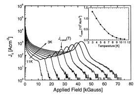
Fig. 3.  $J_{\rm c}$  vs. field determined from the global magnetization curves for temperatures between 3 and 11 K. A pronounced peak-effect at high fields, close to  $B_{\rm c2}$ , indicates the existence of residual bulk pinning in YNi<sub>2</sub>B<sub>2</sub>C over this temperature range.  $J_{\rm c-peak}$  (inset) increases continuously with decreasing temperature.
