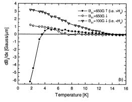
Fig. 2. (a)  $dB_z/dx$  vs.  $B_s$  for field profiles similar to those shown in Fig. 1(b,c) at 7.5 K (top panel) and 2 K (bottom panel). Clockwise (anticlockwise) direction of the loops is due to surface and geometrical barriers (bulk pinning). (b)  $dB_z/dx$  vs. temperature for increasing (solid symbols) and decreasing (open symbols) applied field at 100 G (triangles) and 650 G (circles), lower and greater than  $H_p$ , respectively, over this temperature range.
