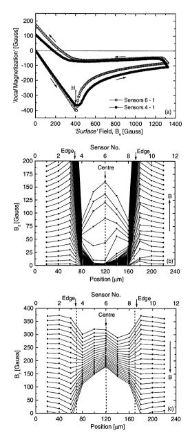
Fig. 1. (a) Local magnetization  $(B_z - B_s)$  vs.  $B_s$  for sensors positioned at the sample centre (6) and edge (4) of a platelet  $YNi_2B_2C$  crystal at a temperature of 7.54 K. (b, c) Field profiles measured directly for increasing (b) and decreasing (c) applied field.
