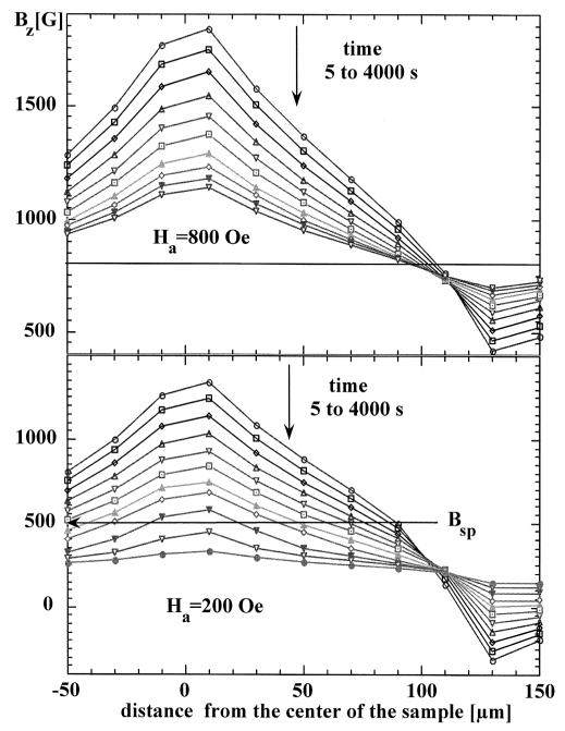
Fig. 2. Decay of the magnetic induction recorded by the Hall array placed on the surface of the BSCCO crystal, after field cooling from 30 to 14.8 K in a field 3 kOe higher than the target field, followed by rapid quenching of the field to 800 (upper panel) and 200 Oe (lower panel).
