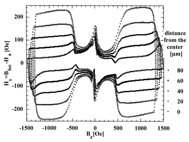
Fig. 1. Local magnetization loops recorded at 20 K on BSCCO crystal with ramp rate of 1.3 Oe/s. At  $B_{\rm sp} \approx 500$  G, an abrupt increase of the width of the hysteresis loop and the appearance of a field gradient in the bulk of the sample marks the crossover from a surface barrier-supported screening current to pinning in bulk.
