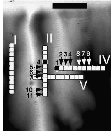
Fig. 3. Zoom of Fig. 1 indicating some of the pairs of probes between which avalanche correlations were measured. The probes indicated by black dots were the “fixed” members of the set of pairs under study within a given arrangement (see text). The scale bar is 0.15 mm long. Probes not indicated by arrows were not working properly at the time of the correlation experiments, so they were not used.
