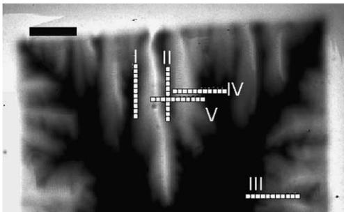
Fig. 1. Micro-Hall probe arrays on the flux penetration landscape. A MO image of approximately half sample area is shown at an applied field of 450 Oe at 4.8 K, on which the different locations of the micro-Hall probe arrays are indicated by white dots. As the magnetic field is increased, all the “ridges” observed in the magnetooptical picture grow gradually on a macroscopic scale. The scale bar is 0.2 mm long.
