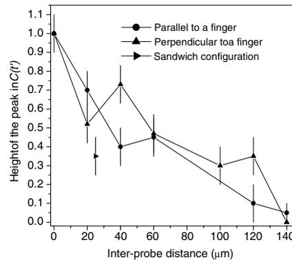
Fig. 4. Correlation results at 4.8 K for pairs of probes with different spatial configurations (see text and Fig. 3). Note that the centers between two consecutive probes within an array are 20  $\mu\text{m}$  apart, and that the sample is 25  $\mu\text{m}$  thick. The experimental misalignment along  $x$  and  $y$  of the two probes in the sandwich configuration, is estimated to be less than 30  $\mu\text{m}$ .
