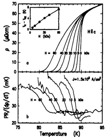
Fig. 1. The resistive transition (a) and the normalized photoresponse (b) of YBa<sub>2</sub>Cu<sub>3</sub>O<sub>7- $\delta$</sub>  epitaxial film at various magnetic fields. Inset: the nonequilibrium PR onset temperature,  $T_{NE}$ , as a function of H.
