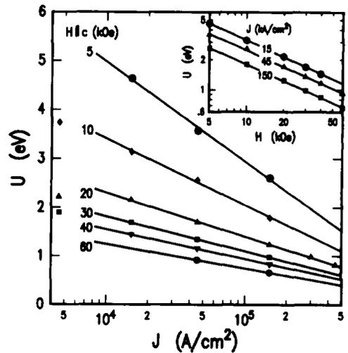
Fig. 3. The activation energy,  $U(0,H,J)$ , as a function of current density and magnetic field as obtained from the fit of the experimental data to  $U(t,H,J) = U(0,H,J)(1-t^2)(1-t^4)^{1/2}$ . The lines emphasize the logarithmic dependence of  $U$  on  $J$ , and the power law dependence on  $H$ . The slopes of the lines in the insert are 0.88, 0.81, and 0.76 for current densities of 15, 45, and 150  $\text{kA/cm}^2$  respectively.
