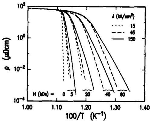
Fig. 2. Arrhenius plot of the resistivity at several representative values of magnetic field and current density.
