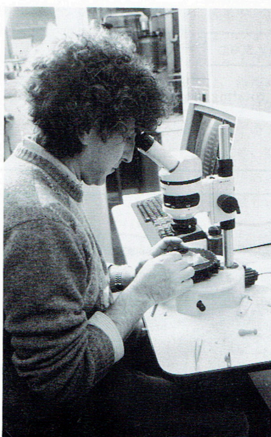
Fig. 4 The low temperature crystal mounting technique is shown using a low power stereo microscope coating the crystals with a viscous oil in the crystallization droplet. After all mother liquor solution covering a crystal is removed, it is picked up with a thin glass fiber, and then placed directly in the stream of cold N_2 to shock freeze it (2),(3) . It should be emphasized, that the crystal is mounted without putting it in a capillary .
