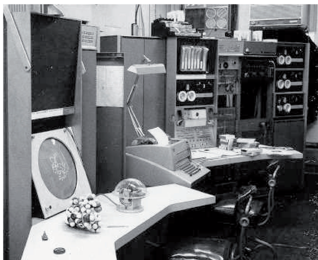
Figure 5. Image of the Kluge, one of the earliest (if not the earliest) molecular graphics systems, which was developed by Cyrus Levinthal at MIT in the early 1960s. The computer was a Digital Equipment Corp. (DEC) PDB-7, and the glass hemisphere was a powerful interactive device that permitted rotation in three dimensions.
