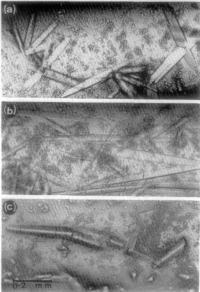
FIG. 2. Development of cracks with crystal growth. Crystals have been obtained as described by Yonath *et al.* (1982a) from 30% methanol at pH 8.4, and are shown after; (a) 25 and (b) 40 days of growth. (c) Cracked crystals which have been grown from a mixture of 17% (v/v) ethylene glycol and 17% methanol (pH 8.4).
