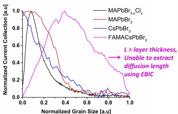
**FAMACsPbBr<sub>3</sub> forms a junction resembling a p-i-n junction while with the other films a p-n junction forms**
