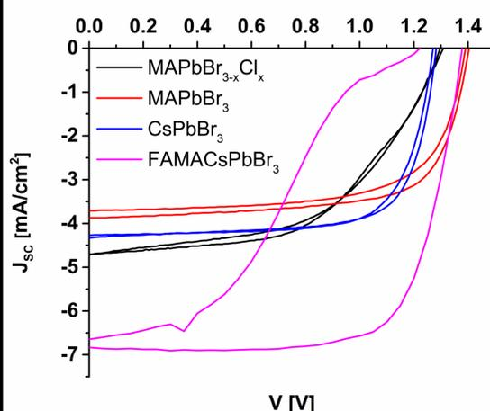
**Unlike the single cation devices, FAMACsPbBr<sub>3</sub> has a strong hysteresis in the device I-V characteristics**
