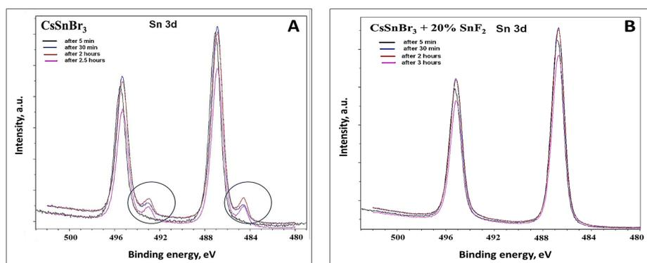
Time-dependent XPS analysis shows that pristine CsSnBr<sub>3</sub> is susceptible to beam-damage (metallic tin formation is observed within ~0.5 h of continuous X-irradiation; Fig. A).
