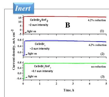
Devices maintain most of their initial photocurrent, if measured in inert atmosphere (with white LED, ~2 sun intensity) (Fig. B (1) and (2)), and are stable for 5 h.
