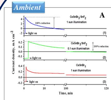
Strong reduction in the photocurrent density (Fig. A (1) and (3)) of the cell is observed, when measured in ambient atmosphere (~65% RH with 1 sun intensity).
