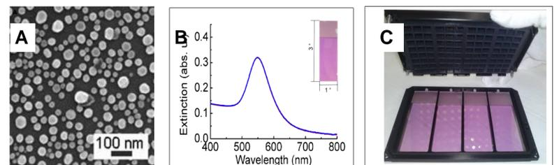
Basic LSPR transducer. (A) High-resolution scanning electron microscope image of a 5.0 nm (nominal thickness) Au island film prepared by evaporation on a glass microscope slide followed by annealing 10 h at 580 °C. (B) Transmission UV-Vis spectrum, presenting the localized plasmon absorption band of the LSPR transducer; inset: photograph of the transducer (1"×3"). (C) The Microplate Microarray from Arrayit Corp., USA.
