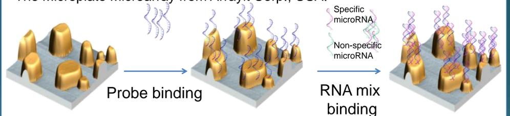
Schematic representation of the miRNA assay. The Au island based LSPR transducer is functionalized with a SAM of covalently attached thiolated DNA having a sequence complementary to the target miRNA, followed by incubation with samples containing miRNA strands.
